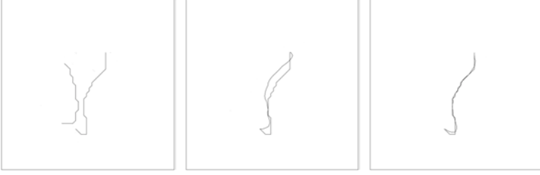
Fig. 1. Left panel: The two curves to be matched. Middle panel: The position of the curves after matching the end points. Right panel: The final result of matching the two curves.
